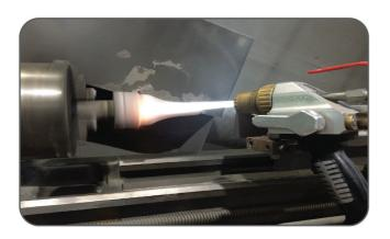
We work with the world's leading thermal spray coating powder producing companies. We have the thermal spray powders which we use in our production produced as a special mixture (Tungsten, Cobalt, Chrome, Nickel, Borone) We are able to do thermal spray surface coatings from 30 HRC up to 65 HRC.
